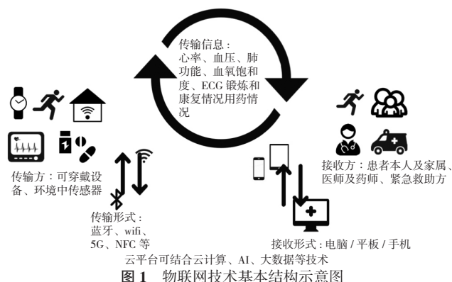
Figure 1 Schematic diagram of the basic structure of IoT technology
